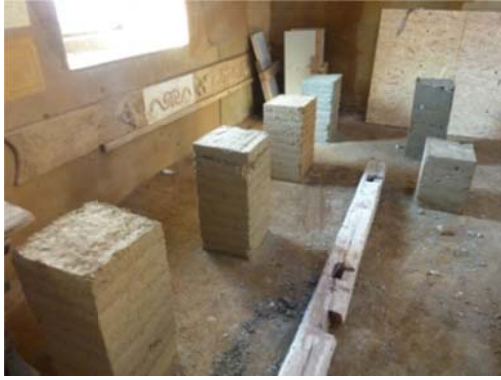
Picture 3: Create rammed earth of test pieces
